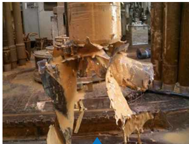
The FM 116L 5,75" Magnum Fishing Magnet® being used after a milling job after milling
